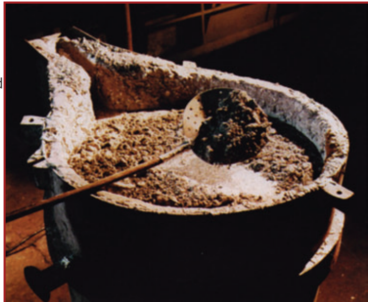
This photo shows dry dross being removed from a transfer ladle after F1/RD treatment. Dry dross reveals minimal aluminum content in the dross.
